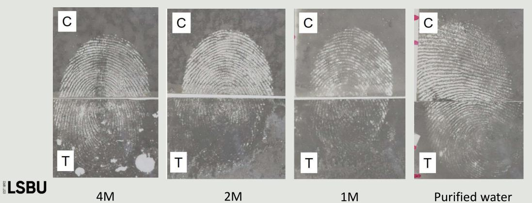
• Silver VMD on PET after exposure to potassium hydroxide (10<sup>th</sup> depletion)
