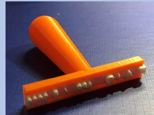
3D printed model adhered to handle
